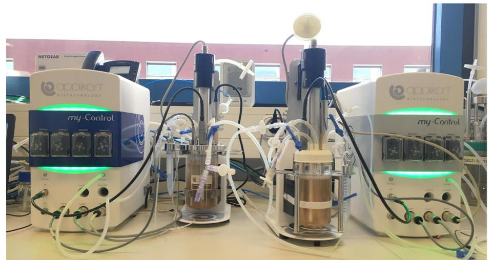
**Figure 2:** Experimental reactor setup with miniBio (left) and Appliflex ST (right) bioreactors.
